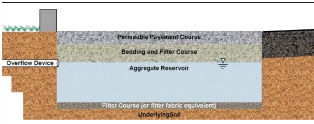
Figure XIV.1: Schematic Diagram of Permeable Pavement without Underdrains
